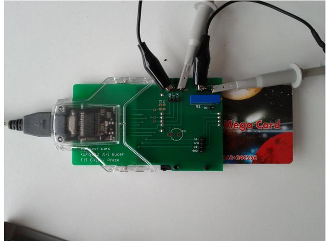
Figure 3. Smart card connected to the card reader through the interface HW board
