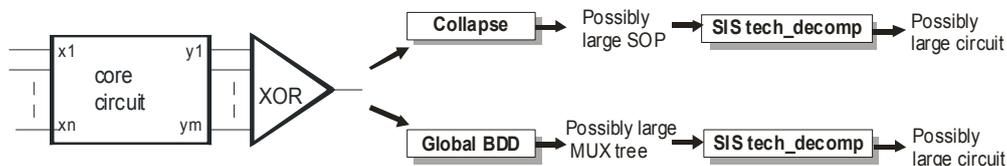
Figure 4: Parity benchmark circuits construction
