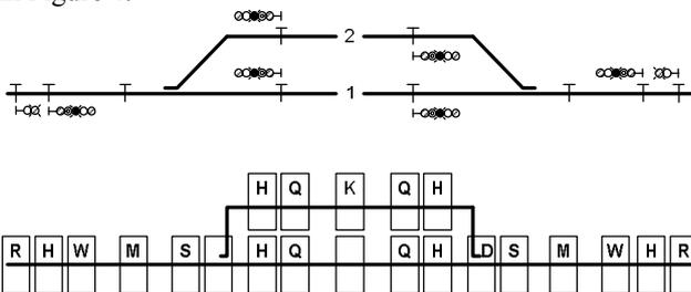
Figure 3. Simple railway station with relay-based blocks
