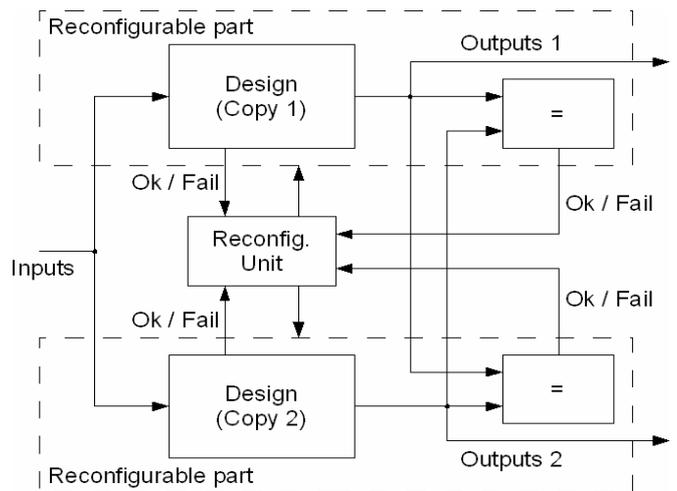
Figure 2. Block diagram of Modified Duplex System (MDS)
