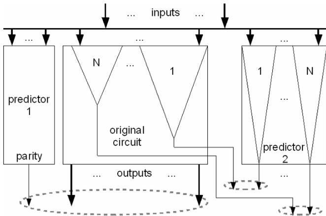
Figure 7. Block diagram of “Complete” design
