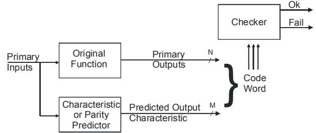
Figure 1. Basic Concurrent Error Detection diagram
