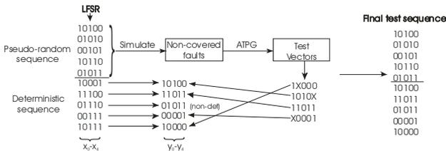
Figure 5: Test sequence generation
