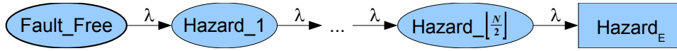
Fig. 6. Dependability model of generic N-modular redundant system used to calculate exact failure distribution function.
