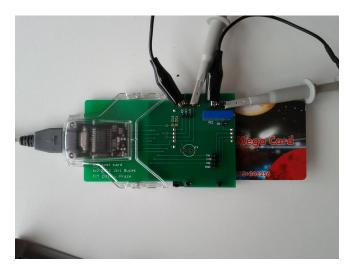
Figure 3. Smart card connected to the card reader through the interface HW board
