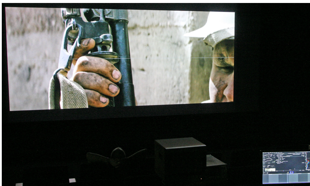
Figure 3.2: An example of receiver synchronization without frame alignment demonstrated with Sony SRX 4K projector. (Note the white line in the middle of the screen.)
