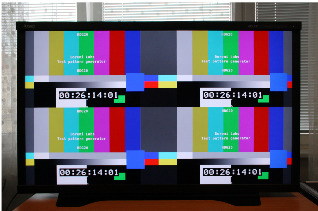
Figure 2.2: A 4K image displayed on a 4K LCD Monitor (Astro Design DM-3400) in the CESNET laboratory. The four 2K HD-SDI quadrants can be clearly seen.
