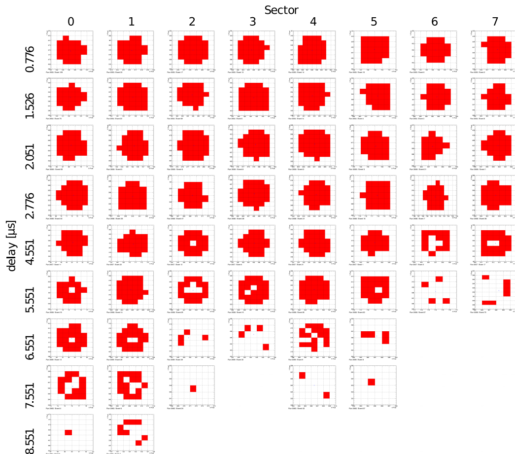
Figure 5.19: Typical proton clusters for each sector and different delay between the PMT trigger signal and the start of data acquisition. Source: [A.9].
