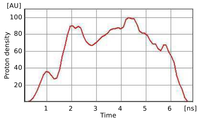
Figure 5.8: Simulated time distribution of proton density in a cyclotron bunch for the energy 34.8 MeV. The corresponding bunch period (cyclotron frequency) is 38.8 ns (25.8 MHz). Credit: [106].
