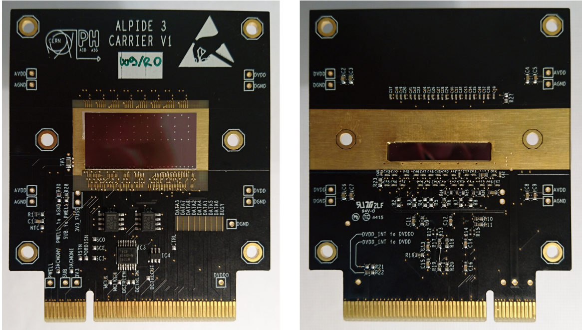
Figure 5.14: 3 rd prototype version of the ALPIDE chip placed on a carrier board. On the left-hand side is a front view of the carrier board with the chip bonded in the middle of it. On the right-hand side, there is the back side of the same carrier board with a technological hole in it, located under a part of the chip. The hole was utilized for measuring false proton hits (see text for details).
