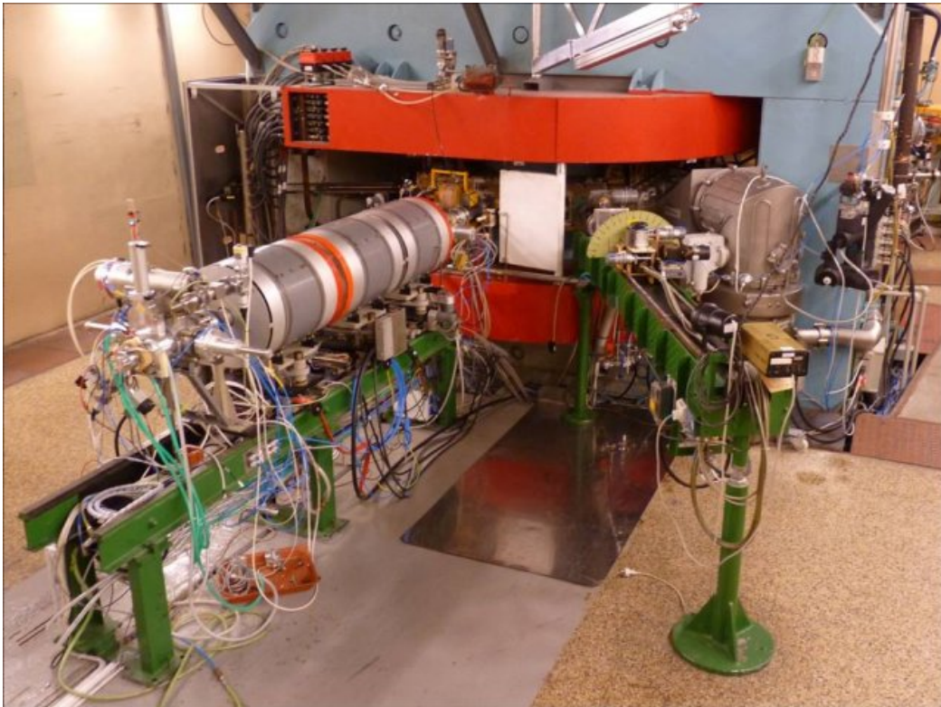
Figure 2.21: The U-120M cyclotron in NPI Řež. On the left-hand side we can see the beam pipe for the negative mode with focusing magnets around it. Credit: [47].
