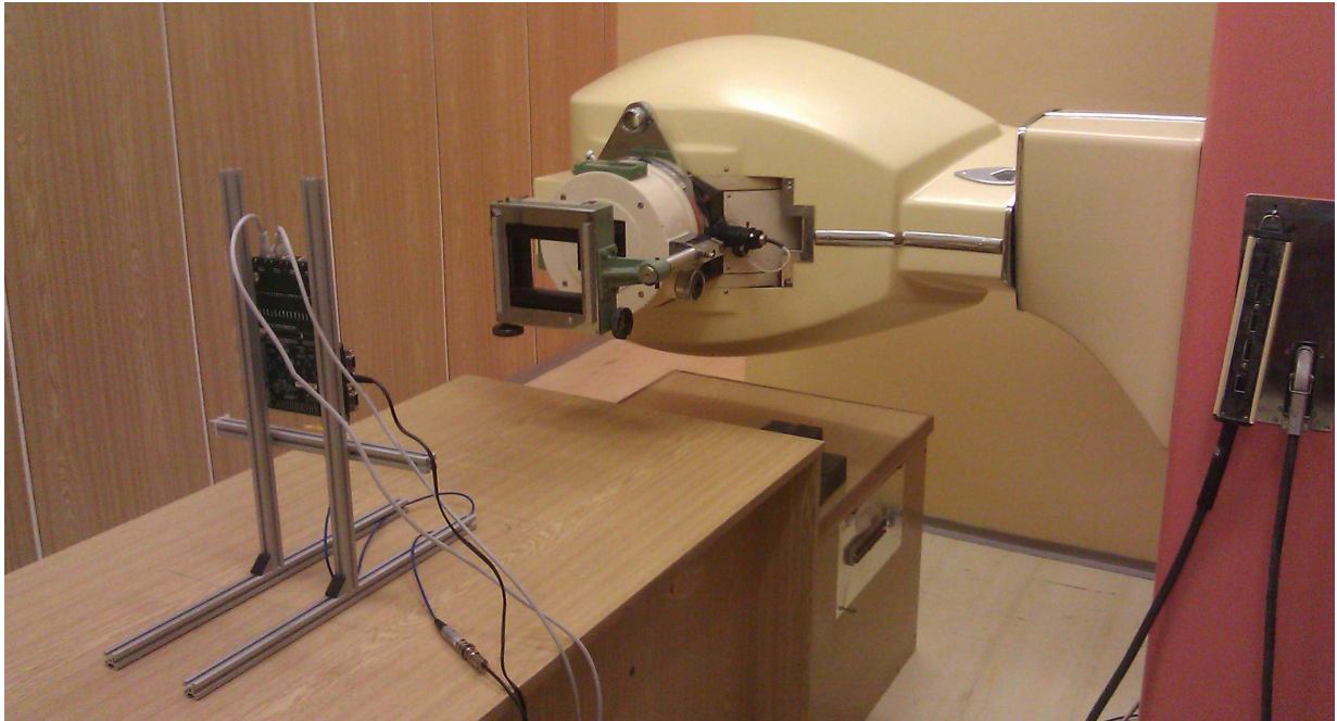
Figure 2.29: Picture of the gamma irradiation apparatus with an irradiated target (FPGA board) in front of it.
