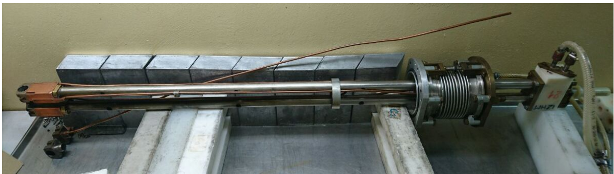
Figure 2.25: Ion source of the U-120M cyclotron, used for the negative acceleration mode. The plasma chamber is on the left-hand side.
