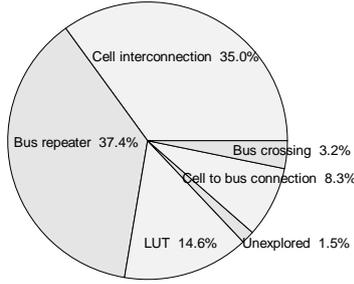
Figure 3: Distribution of the s1488 bitstream according to FPGA resources, where a fault modifies the design
