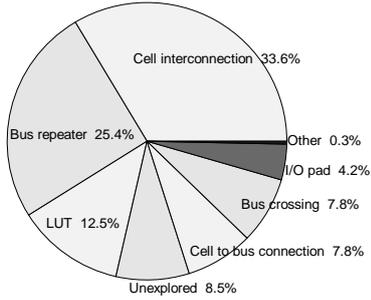
Figure 2: Resources in AT40K Bitstream. *IO pads* and *others* were not tested, *forbidden* are not listed
